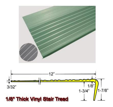
Light-Duty Vinyl Stair Treads boast raised horizontal ribs which provide excellent traction and a stylish appearance. The raised rib pattern allows dirt and moisture to fall between while maintaining traction.
